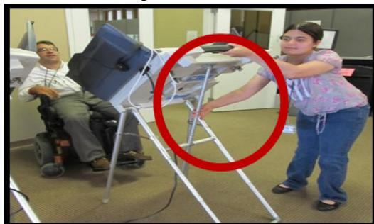
If the voter complains of glare on the screen or requests the screen be tilted, adjust the screen by pushing the button on the back bar and lifting the screen up
