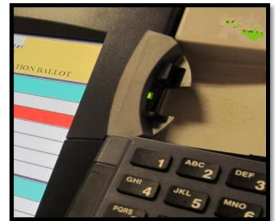
To start the voting process, insert the voter's card into the slot shown here.
